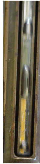
Fig - 10. Slug flow
