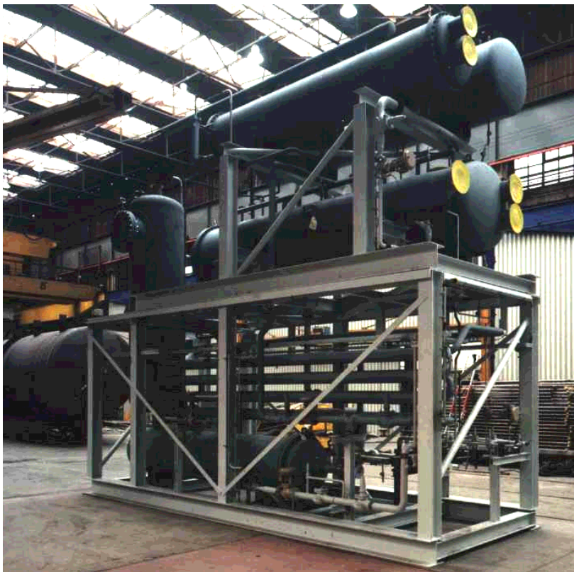
Figure 7 Diagram of the ARP on the manufacturers facilities during pressure tests.
